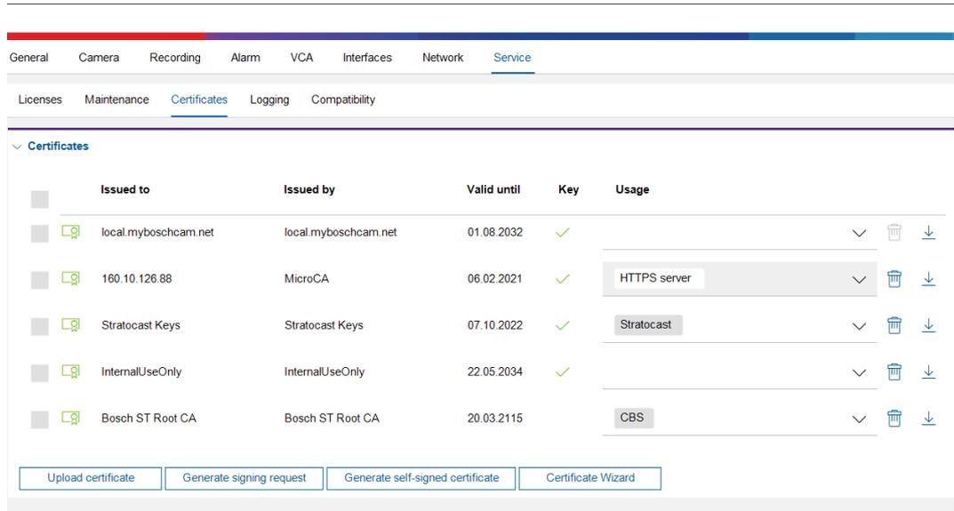
15. Restart the device. After the restart, the newly created signed certificate will apply as a TLS communication encryption certificate.
