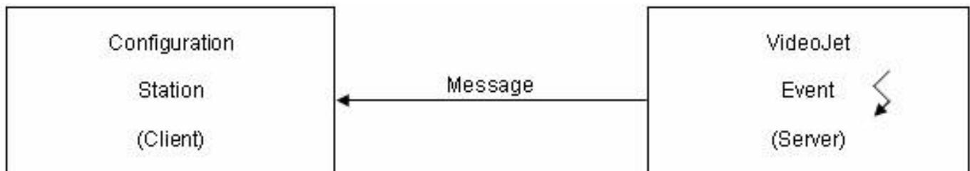
RCP is capable of sending messages on certain events. Before an RCP client can receive these messages, a registration at the VideoJet is necessary.
