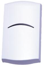
The wLSN Relay Module allows the control panel to switch outputs wirelessly by turning on or off a Form C relay. The wireless Local SecurityNetwork (wLSN) protocol allows multiple output devices, including the wLSN Relay Module, to be synchronized so that they all operate together using the same cadence. The wLSN Relay Module also accepts a supervised sensor loop input from an external device.
