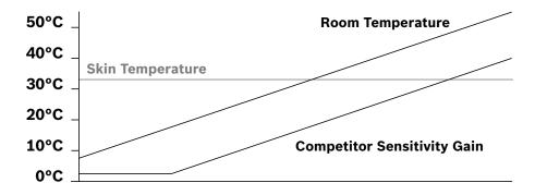
With Professional Series detectors, the sensor gain increases as expected – but only until the room temperature reaches 33.3°C (92°F). Using two PIR sensors with multiple high-quality lenses, Bosch increases the signal-to-noise ratio within that narrow temperature band. Once the room temperature exceeds the surface temperature of an intruder, the sensor gain decreases again, minimizing false alarms.
