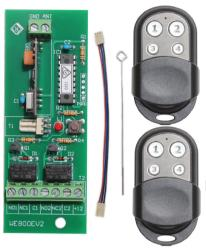
The WE8000EV2KIT is an RF arming kit that is designed to provide a convenient ON / OFF control for the Solution 8xx and Solution 2000 / 3000 / 4000 series control panels. Provision is available for the control of up to two external devices via the onboard relays.
