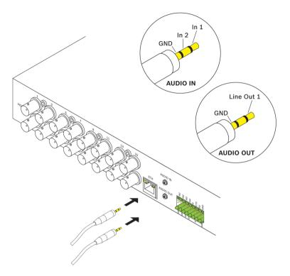
The unit has two audio ports for audio line signals.
