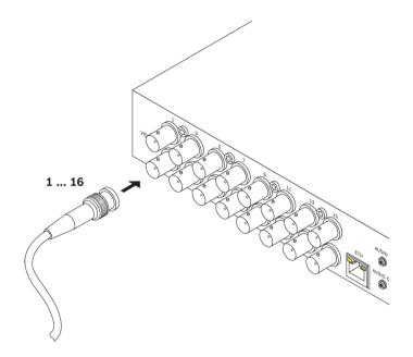
You can connect a maximum of 16 video sources to the VIDEOJET multi 4000 encoder. Any cameras and other video sources that produce a standard PAL or NTSC signal are suitable.
