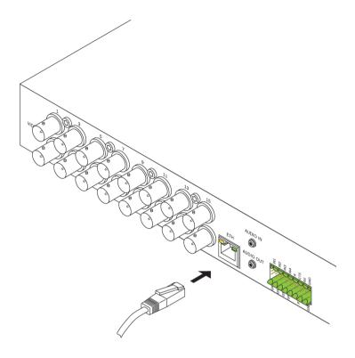
You can connect the unit to a 10/100/1000 Base-T network using a standard UTP category 5 cable with RJ45 plugs.
