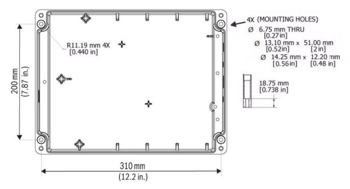
Figure 5.1: Dimensions, mounting holes, VIDEOJET connect 7000
