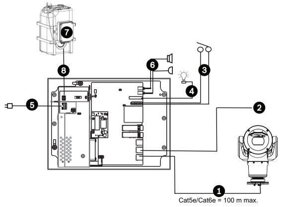
Figure 3.1: Basic configuration with VIDEOJET connect 7000
