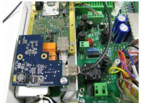
Figure 5.2: Fiber optic module installed in MIC IP PSU
