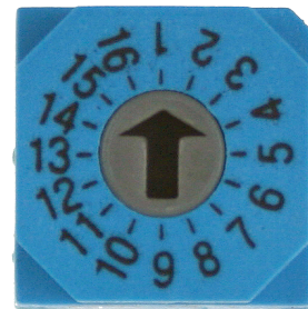
Figure 24: Rotary Switch Address Settings
