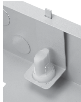
Figure 2: Tamper Bracket Installation
