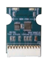
P/N - CM255B Panel Default Unlock Key Will reset Installer PIN and RAS PIN on Solution 6000 panels.
