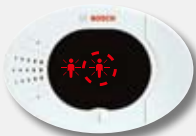
Fire or intrusion alarm (system is off)
