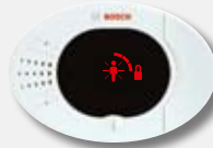
Exit delay in progress
