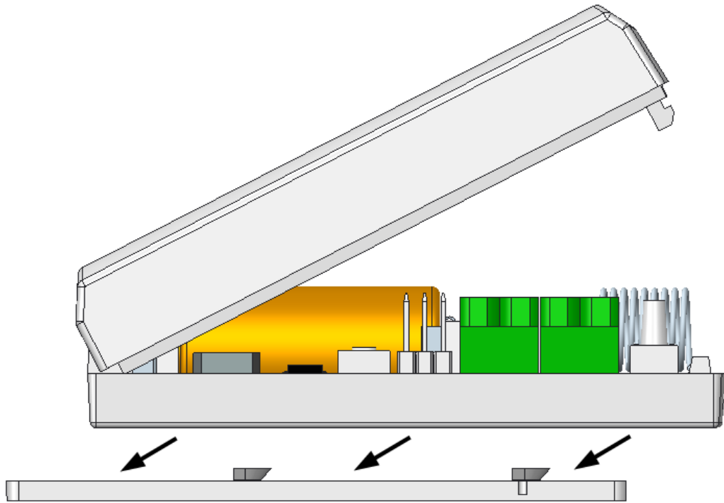
Figure 3.3: Slide point transmitter over base
