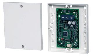
The SE 220 LSNi SmartKey arming device with connectable code keypad/reader is a system solution for arming/disarming intrusion alarm systems. Arming/disarming is carried out by using the SmartKey key then entering the user code.
