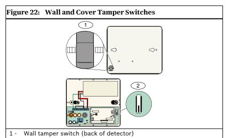
Cover tamper switch (inside of detector)
