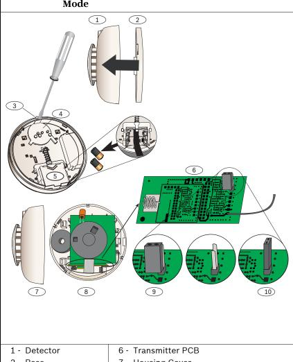
Figure 18: Returning the Smoke Detector to Undiscovered Mode
