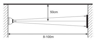
Mount on solid surfaces (structural wall or girder)
