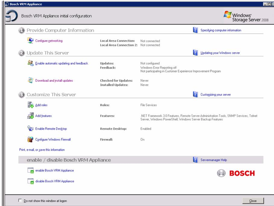
4. The top level view of **Bosch VRM Appliance initial configuration** displays an overview of the system’s configuration and settings. Select the link **Configure networking** to get access to the network configuration. For each network port a separate icon is shown. Select the **Local Area Connection** icon that shows the status **network**, then double-click the icon.
