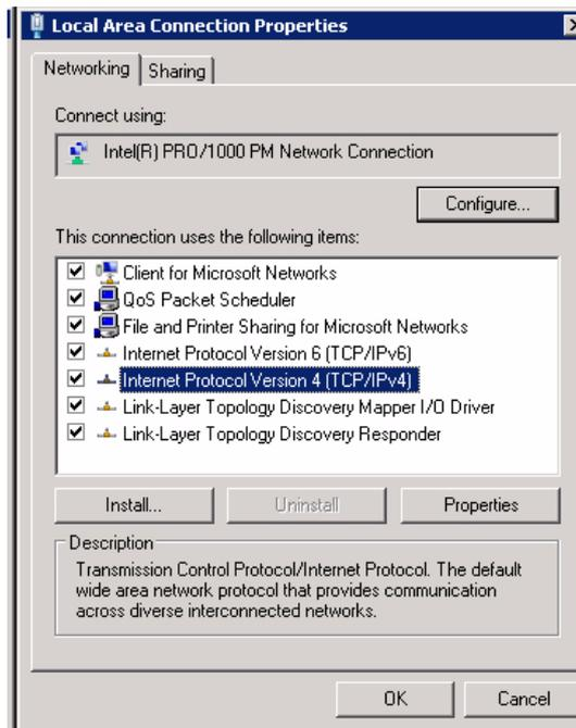
7. This dialog box allows you to set the IP address configuration according to the requirements of your network.
