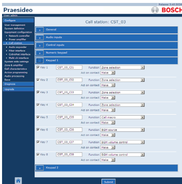
figure 43.29: Configure call station, step 7
