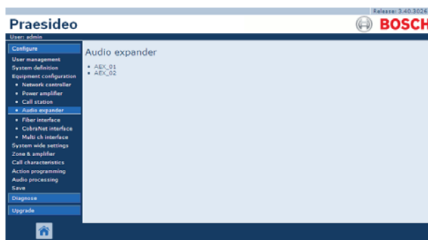
figure 43.30: Configure audio expander, step 1
