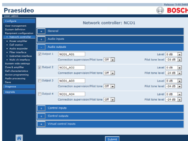
figure 43.6: Configure network controller, step 4
