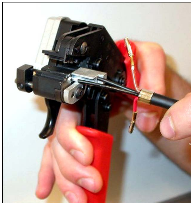
figure 29.16: Cutting a fiber (1)
