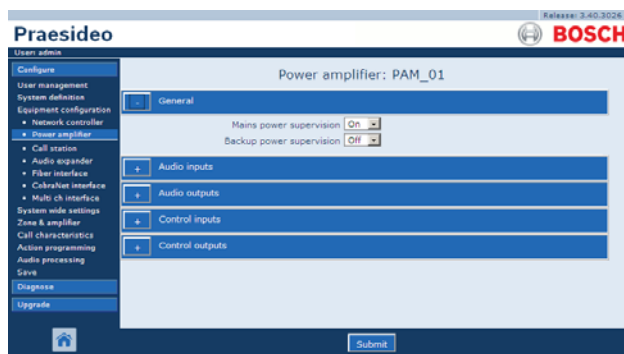
figure 43.12: Configure power amplifier, step 3
