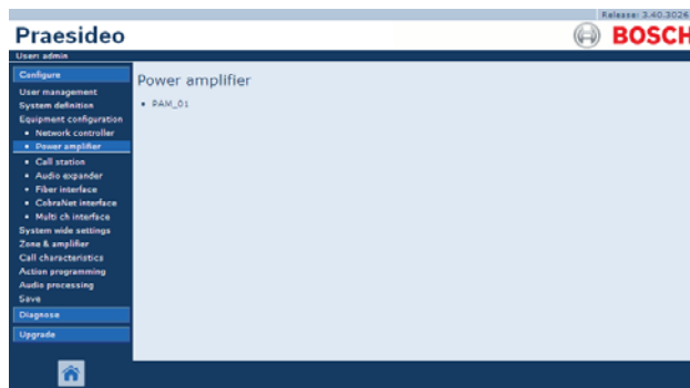
figure 43.10: Configure power amplifier, step 1
