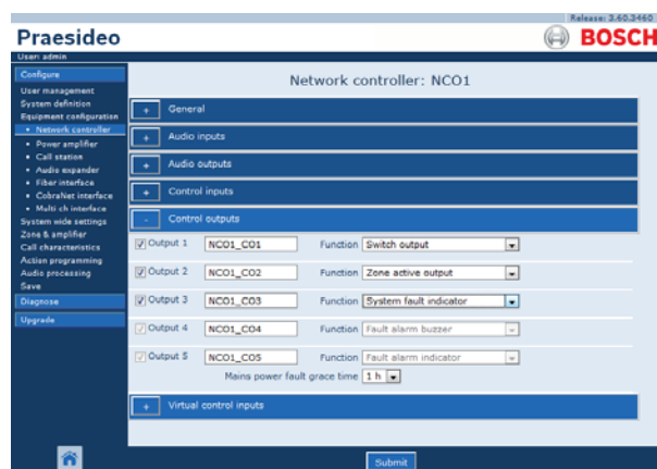
figure 43.8: Configure network controller, step 6
