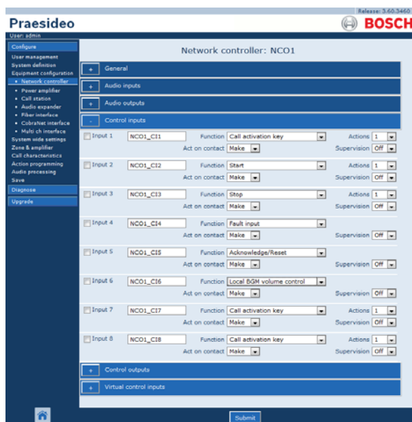
figure 43.7: Configure network controller, step 5
