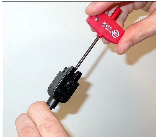
figure 29.37: Tightening the Torx screw
