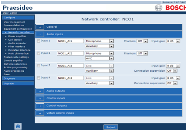
figure 43.5: Configure network controller, step 4
