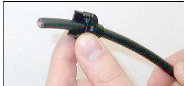
figure 29.6: Back housing on cable
