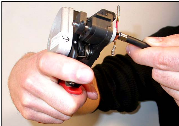
figure 29.18: Cutting a fiber (3)
