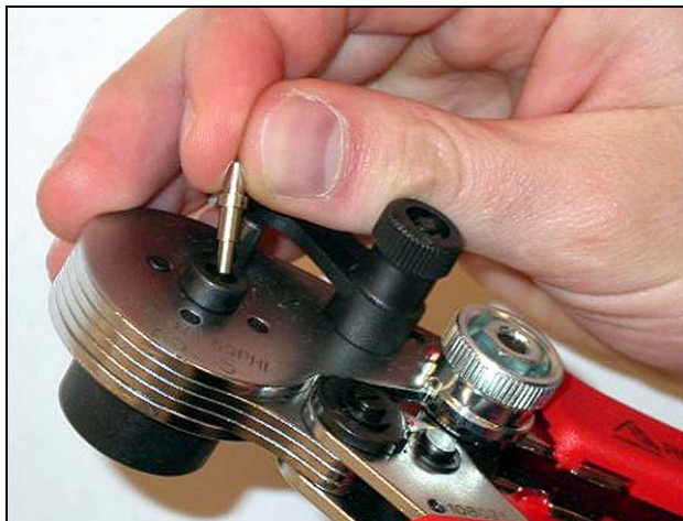
figure 29.21: Inserting a ferrule
