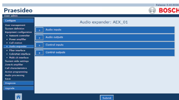
figure 43.31: Configure audio expander, step 2
