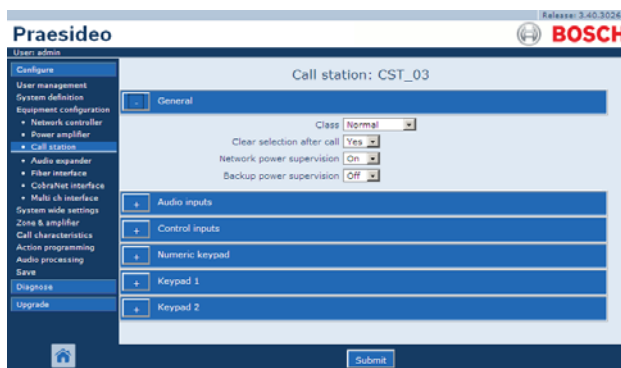
figure 43.24: Configure call station, step 3
