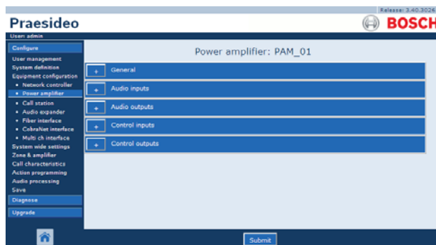
figure 43.11: Configure power amplifier, step 2
