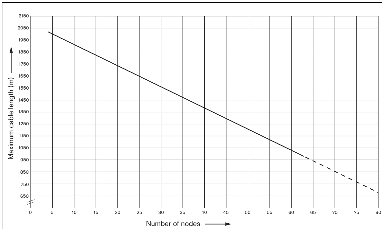
figure 31.5: Maximum optical fiber length vs. number of nodes
