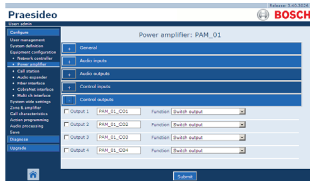
figure 43.20: Configure power amplifier, step 7
