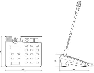
Fig. 2: Dimensions of Call Station
