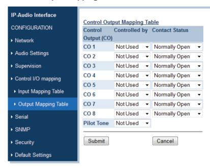
Figure 6.10: Control Output Mapping Table (default)
