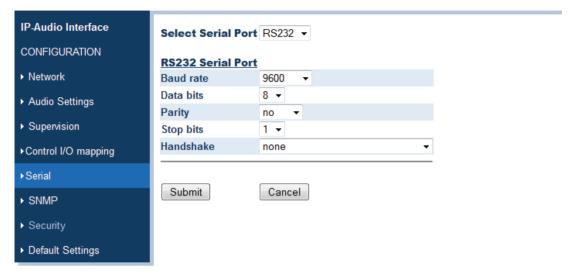
Figure 6.11: Serial (RS-232) screen default
