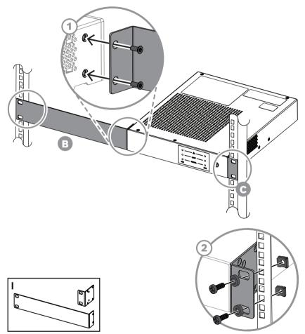
Figure 4.3: Stand-alone mounting in a 19"-rack
