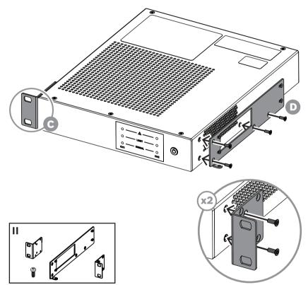
Figure 4.4: Connecting the rack ears and the connecting plate
