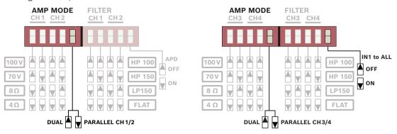
Figure 5.2: Input routing configuration (channel 3 and 4 for PRM-4P600 only)
