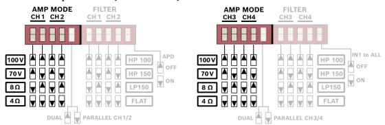
Figure 5.1: Output mode configuration (channel 3 and 4 for PRM-4P600 only)
