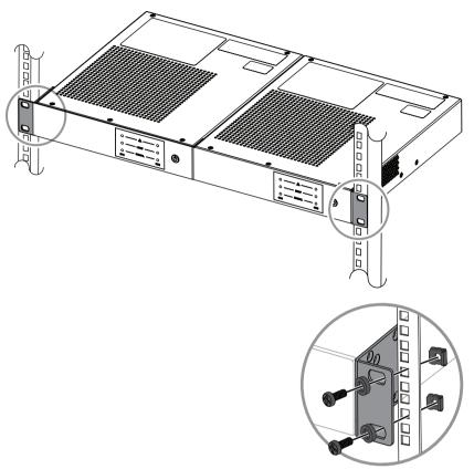
Figure 4.6: Side-by-side mounting in a 19"-rack
