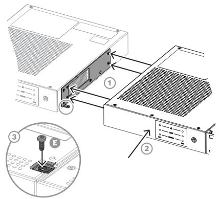
**Figure 4.5:** Two amplifiers hooked together with connection plate mounted and M3 bolt to prevent pushback
