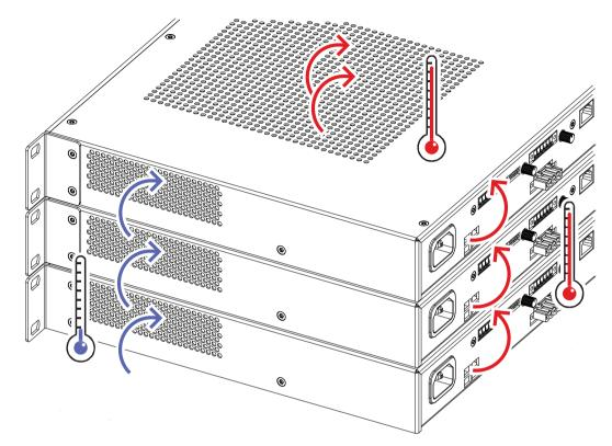
Figure 4.9: Rack mounting of several SYNSONA amplifiers. Illustration of the PRM-4P600 model.
