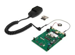
The basic call station kit is an open frame call station to create dedicated full custom operator panels for PRAESENSA Public Address and Voice Alarm systems. It has the same functionality as the PRA-CSLW, but without LCD user interface to facilitate easier mounting in operator desks or in wall-mounted fireman's panel enclosures.
