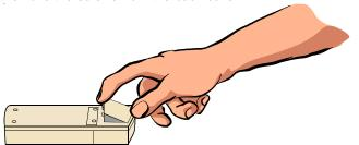
Insert the new battery. Be sure to observe the proper polarity. Close the cover.
