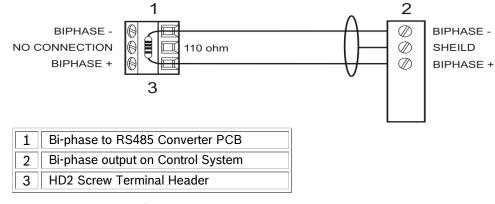
Figure 1: Connections for Bi-phase
