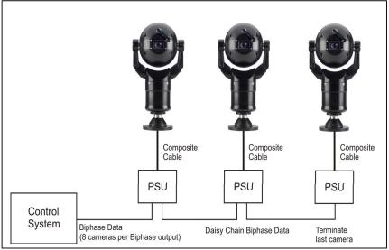
Figure 2: Daisy chain configuration for Bi-phase controller
