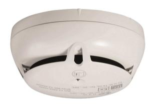
The OOH740-A9-Ex is an Dual-Optical Detector for fire detection in potentially explosive areas in zones 0, 1 and 2. It can be programmed either as a dual-optical or as a thermal detector by inserting defined resistors.
