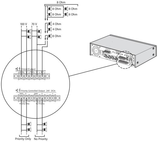
Figure 6.4: Priority input and control terminals
