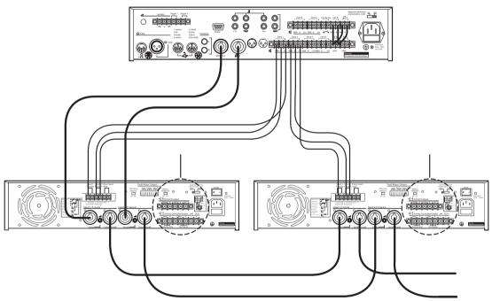
Figure 8.3: LBB1925/10 and power amplifier control terminals example
