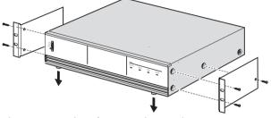
Figure 4.1: Brackets for 19" rack mounting
