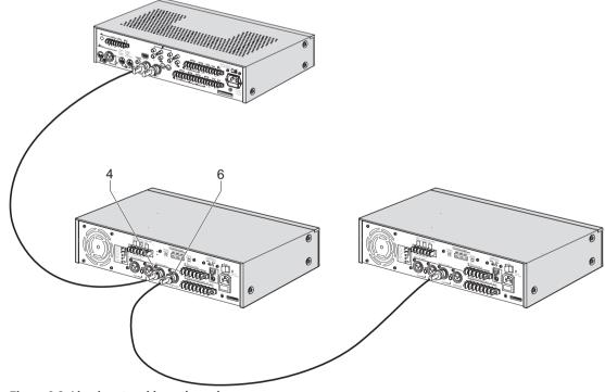
Figure 6.2: Line input and loop-through
