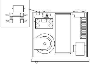
Figure 5.5: Internal fuse settings LBB1930/20, LBB1935/20, LBB1938/x0
