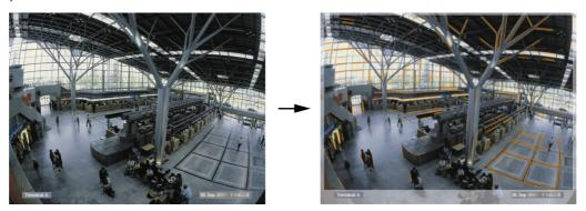
Then click **Estimate Lens Distortion** and verify the result again. The program only adjusts the distortion in the selected area.
