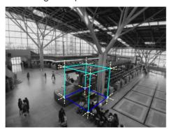
**Note:** The cube was estimated from the main directions of detected straight structures in the image.
