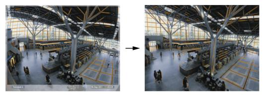
**Figure:** On the right image, the edges are straight. The ceiling lamps and the marking lines on the ground are not distorted.
