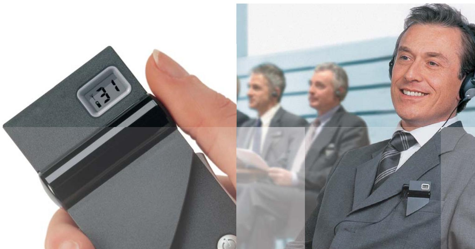
For wireless convenience, Bosch also offers the Integrus, a digital infrared language distribution system that is immune to interference from lighting systems and bright sunlight. It produces crystal-clear sound due a very high signal-to-noise ratio plus built-in error correction.
