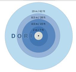
When mounted at a height of 3 m (10 ft) the 180° version of the camera has the following coverage radius for the four levels:
