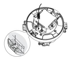
6. Use the supplied screws and washers to securely mount the camera to the surface; if the surface is too thin, use appropriate bolts (not supplied).
