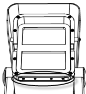
Figure 4.7 3D Diffuser (area circled)
