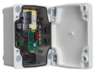
Bosch offers a series of stand-alone power supply units that provide 24 VAC power to AUTODOME 7100i non-IR cameras for applications without PoE or for redundant power applications with PoE. Each unit has a cover door that provides IP rating IP66/ UL Type 4X ingress protection and meets power and electrical safety requirements in extreme environmental conditions. The unique design and the IK10 rating protect the power supply units from vandalism and tampering events.
