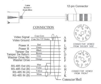
MIC Cable – 12-pin (for all MIC cameras except current thermal cameras)
