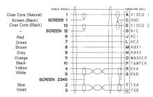
MIC Cable - 14-pin (for current MIC thermal cameras)
