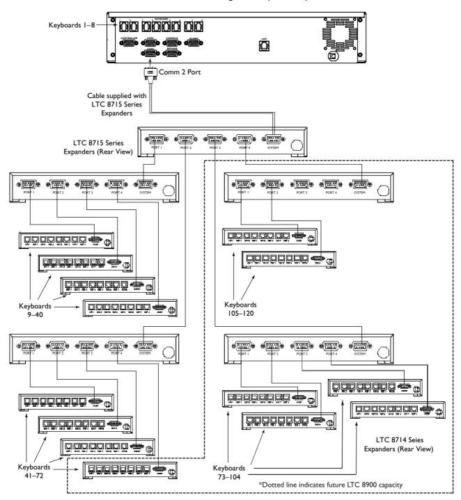
Figure 11 Typical Installation for More than 32 Remote Keyboards
