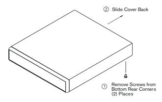
Figure 1 Top Cover Removal
