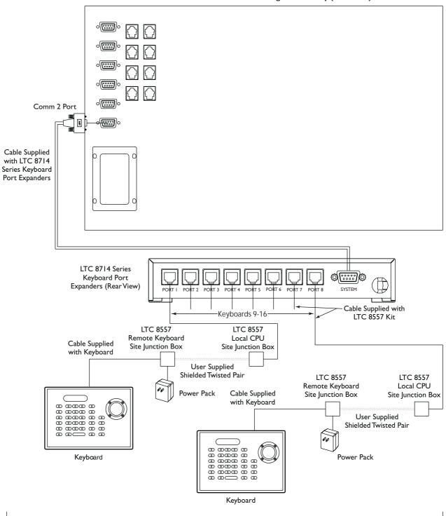
Figure 9 Typical LTC 8714 Series Keyboard Port Expander Application
