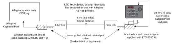
Figure 5.4 Typical Configuration using fiber optic link
