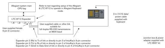
Figure 5.7 Configuration using LTC 8712 Series Console Port Expander
