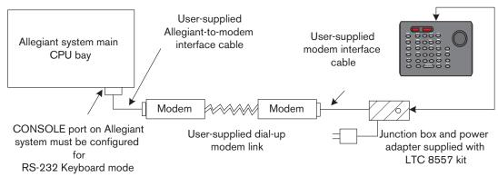
Figure 5.6 Connection Using Dial-up Modem Link
