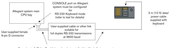
Console pin 2 (Rx) to Tx of link or directly to pin 3 of IntuiKey's 9 pin connector Console pin 3 (Tx) to Rx of link or directly to pin 2 of IntuiKey's 9 pin connector Console pin 7 (Gnd) to Data Gnd of link or directly to pin 5 of IntuiKey's 9 pin connector
