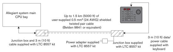
Figure 5.3 Typical Configuration using optional LTC 8557 Series Hookup Kit
