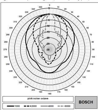
Fig. 7: Vertical polar diagram (high frequency part)
