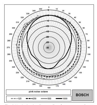
Fig. 6: Vertical polar diagram (low frequency part)
