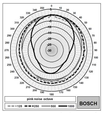
Fig. 4: Horizontal polar diagram (low frequency part)
