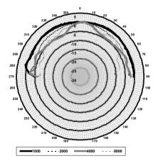
LC4-UCxxE horizontal/vertical polar diagram (low frequency). Normalized at 0-degrees axis.
