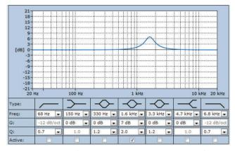
LC3-UC06E specified active equalization required for EN 54-24
