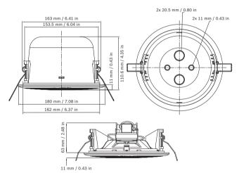
Mechanical diagram LC3-UC06E and LC3-CBB
