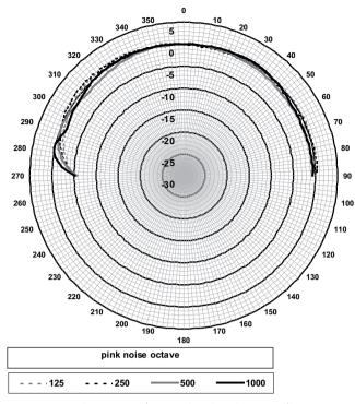
LC3-UC06E horizontal/vertical polar diagram (low frequency). Normalized at 0-degrees axis
