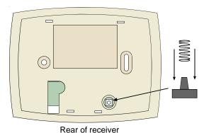
Figure 4 - Installing the Tamper Spring
