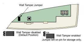
Figure 3 - Wall Tamper Jumper
