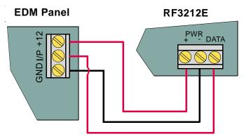
Figure 7 - Connecting to the EDM Panel
