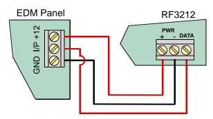
Figure 7 - Connecting to the EDM Panel
