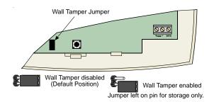
Figure 3 - Wall Tamper Jumper
