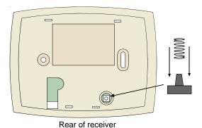
Figure 4 - Installing the Tamper Spring
