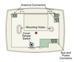
Figure 5 - Receiver with Outer Cover removed
