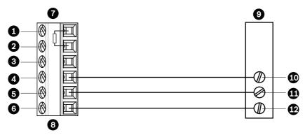
Figure 3.4 Connections for RS232 Operation
