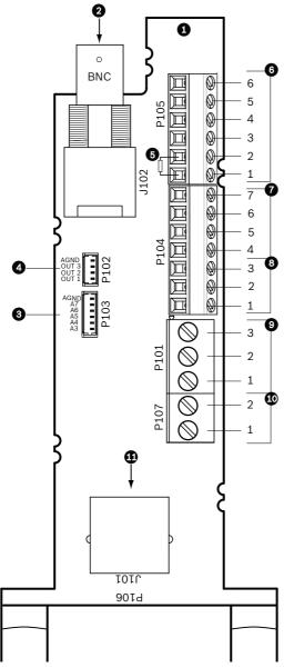
Figure 2.9 Pipe Interface Board Connections
