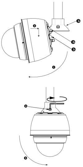
Figure 2.12 Pendant to Roof / Pipe Mount Attachment
