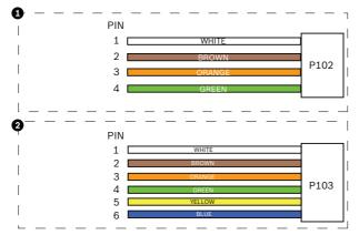
Figure 2.10 Alarm and Relay Connector Plugs
