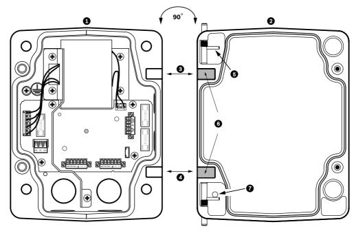
Figure 2.2 Align Cover Door Hinge to Power Box
