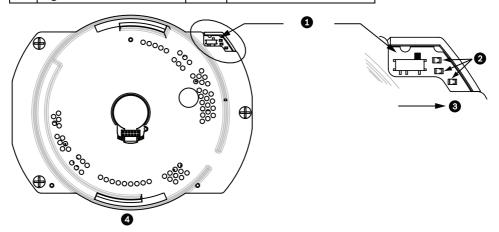
Figure 3.7 Position of CPU Switch for RS485 Operation (camera module not shown for clarity)
