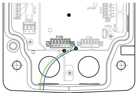
Figure 3.8 Detail of P106 Connections
