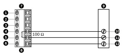
Figure 3.6 Connections for RS485 Operations
