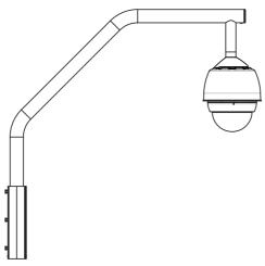
Figure 2.5 Parapet Roof Mount
