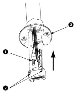
Figure 2.11 Pipe Interface Board to Dome Cap Assembly
