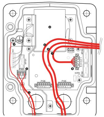
Figure 2.3 VG4-A-PSU1 or VG4-A-PSU2 Power Supply Box
