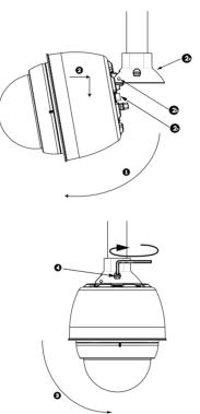
Figure 2.9 Pendant to Pipe Mount Attachment
