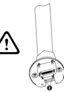
If your pipe mount contains these pins, **DO NOT** attempt to mount a Pressurized Environmental Housing to this mount. You must order the VG4-A-9543N pipe mount option for the Pressurized Environmental Housing.
