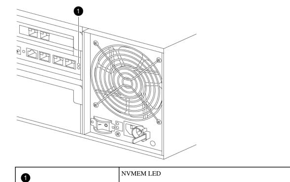
**Note:** The preceding illustration shows a FAS2050 system. The NVMEM LEDs are in a similar location on a FAS2020 or FAS2040 system. The Platform Monitoring Guide contains additional information about the NVMEM LEDs.
