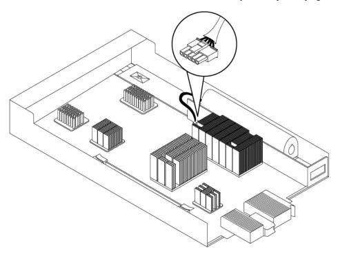
2. Lift the battery out of the holder and controller module.
