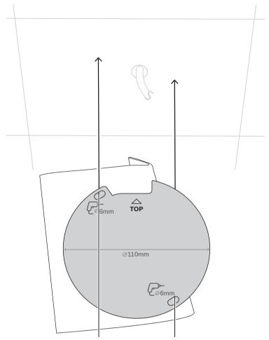
Use an appropriate size drill to mark the holes using the mounting template.
