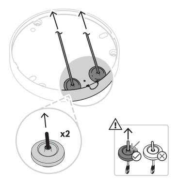
Connect the network cable to the network connector in the camera.
