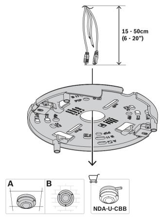
3. Pull the cable through the center hole of the mounting plate. Note: If the cable is not coming out the wall, but along the wall, then the mounting plate needs to be installed in line with the cable. That way the cable won't come through the center hole. The mounting plate has one side available for side entry of a cable. Remove the door on the camera base.
