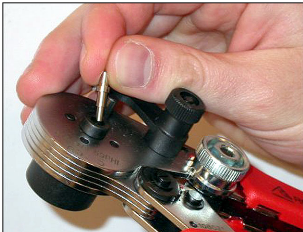
figure 29.21: Inserting a ferrule
