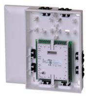
A maximum of 2 IMS-RM Relay Modules can be installed in the ISP-EMIL-120 Expansion Module and in the ISP-EMIL-3RDP Expansion Module if the high power requirement of the connected control elements results in these becoming impossible to actuate directly from the expansion module, or in order to provide dry contacts. IMS-RM Relay Module with 2 relays, 2 switching contacts per relay for dry contacts.
