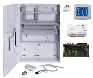
This MAP kit includes one MAP panel 5000 small COM, one MAP Control Center (touch screen keypad), one MAP LSN Gateway Module, one MAP Power Supply 150W and one MAP Panel Enclosure Kit. Using a Bosch Data Bus (BDB) based on Controller Area Network (CAN) technology as the internal and external bus, the panel supports a range of applications as part of the scalable Modular Alarm Platform 5000 system.
