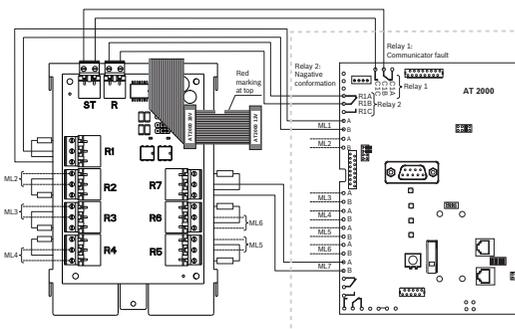
1. The size of the terminal resistors (RE) to be looped in depends on the communicator (for example 10k for the AT 2000).
