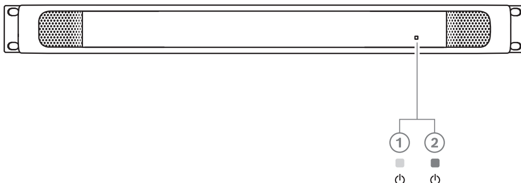
Figure 6.6: OMN-DANTEGTW front panel description
