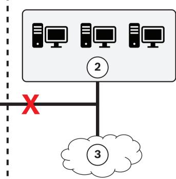
network environment. The Fire Monitoring System has to be part of this exclusive fire alarm Ethernet network without direct access to the Internet (3).
